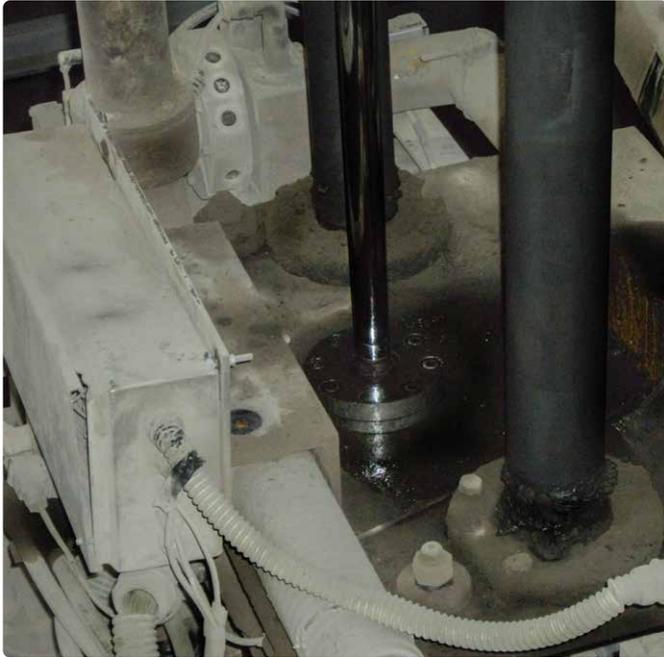
*Example of a poorly maintained CARICAMAT®*
